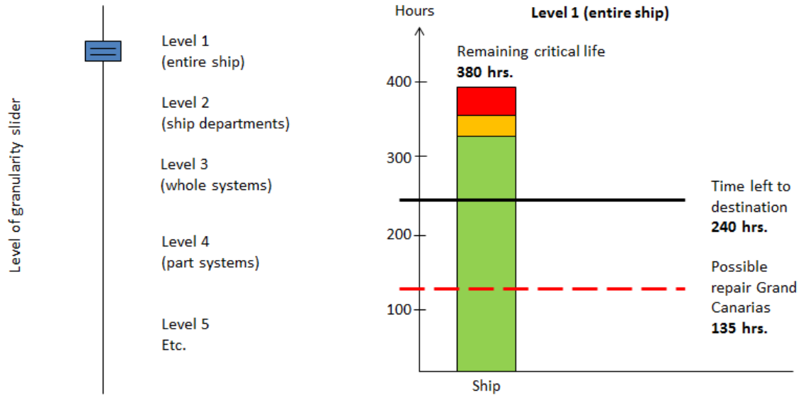
Fig.4: The Ship status indicator screen allows the operator to make an at a glance assessment of the ships present status, remaining life time compared to time to destination or port of repair. The picture shows the top, ship level. By clicking the bar, the operator can open lower levels all the way down to the individual components of the whole ship.
